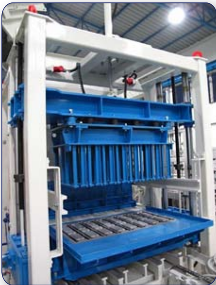
Tamper head bridge
